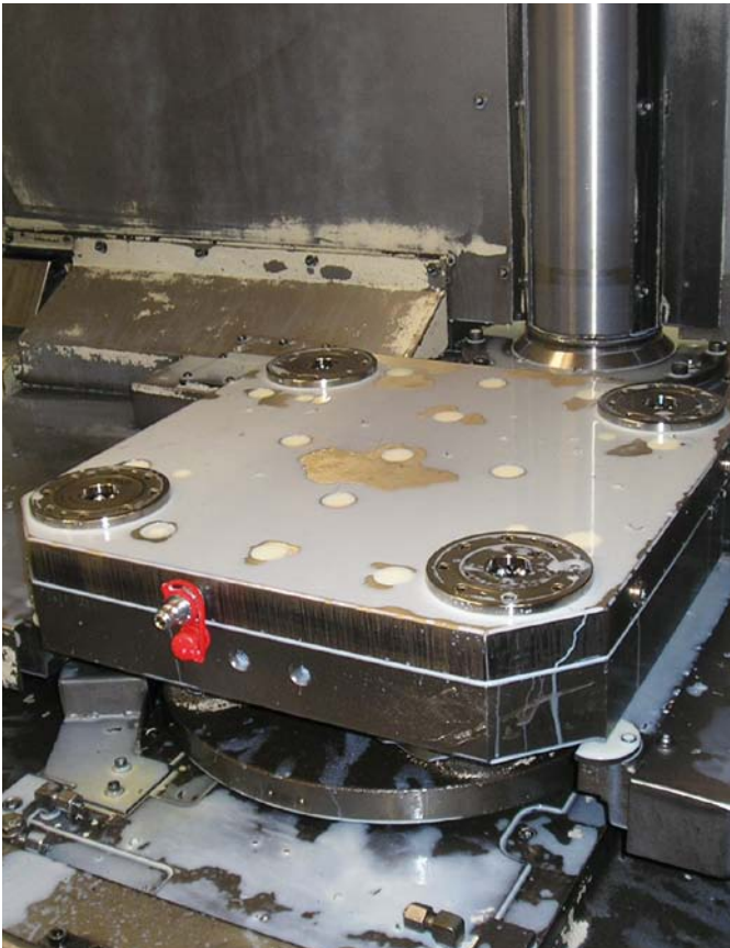
The interior of the clamping module is completely sealed. This means that the system is optimally protected against liquids and dirt.
